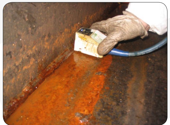
Above & Below: Inspection of a fillet weld using an encoder on-board a weld probe.
