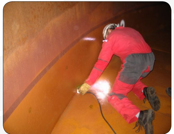
Above & Below: Inspection of a fillet weld using an encoder on-board a weld probe.
