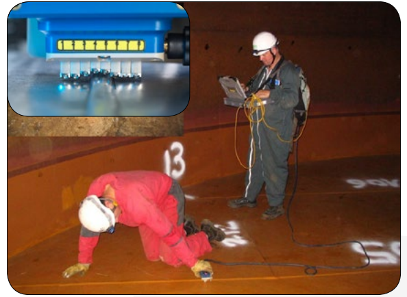
Above: Lap Weld inspection using an adjustable array probe.
